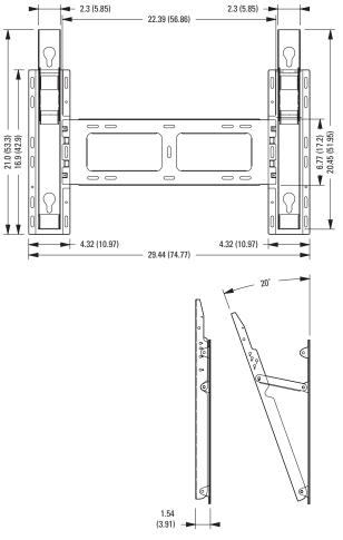
NOTE: VALUE IN PARENTHESES ARE CENTIMETERS, ALL OTHERS ARE INCHES. **Figure 5. PMCP-WMT Dimension Drawing**
